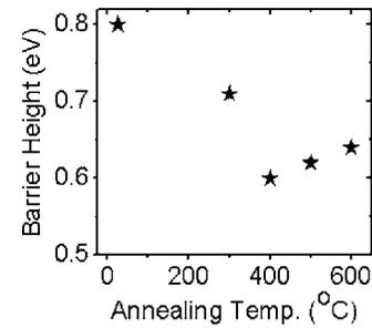
FIG. 2. (Color online) Annealing temperature dependence of the Schottky barrier height.
