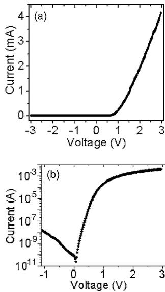
FIG. 1. (Color online) (a) Linear  $I$ - $V$  plot of the diode with as-deposited  $\text{ZrB}_2$  Schottky contact. (b) Semilogarithmic  $I$ - $V$  plot of the diode with as-deposited  $\text{ZrB}_2$  Schottky contact.
